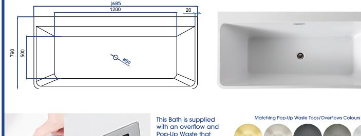
Pop-Up Waste that is tied into the drain waste and is built concealed into the bathtub.
