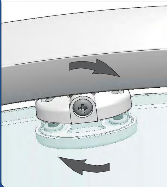
Adjust door heights until doors run smoothly on rails. Adjust door angles so that magnetic seals meet squarely & hold doors in closed position. Turn adjusting screw clockwise to raise door.
