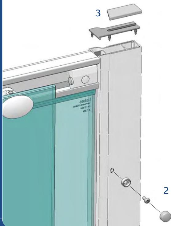
1. Adjust enclosure panels to give even gap to tray edge along both sides, ensure unit is plumb & that doors slide smoothly between stops.
