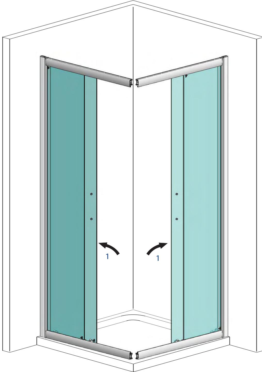
1. Ensuring that 'Top wheels' are at the top, & with doors in fully open position, carefully lift panel sub assemblies onto tray & push fully into wall profiles.
