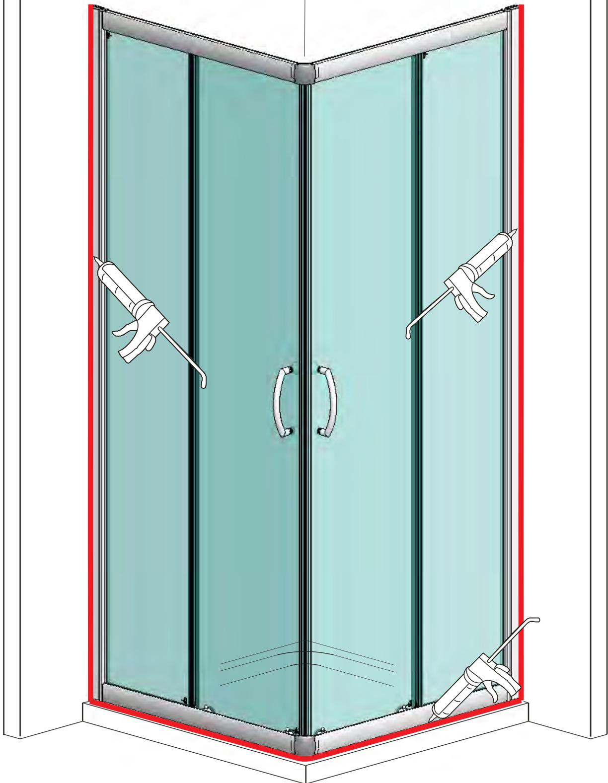
Use of good quality silicone sealant & cleaning / degreasing of all joint areas is recommended.
