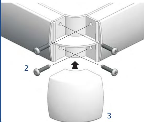
2. Fit corner cleats into open rail ends & secure with 4 x 20 long pan head screws (4 per cleat).
