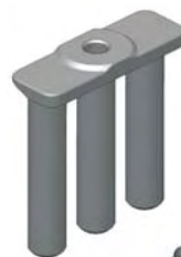
Hinge Boss (Frame 2x) & 3.5 x 12 long self tapping csk head screw(6x)
